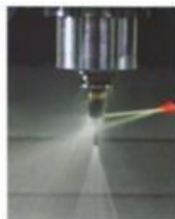
WATER THROUGH SPINDLE HOLE
